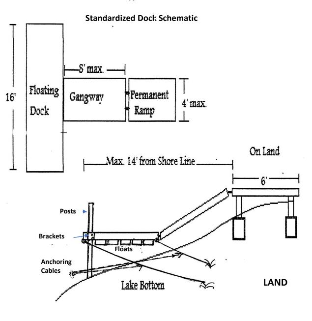
Note: Posts, Brackets and Anchoring Cables are optional if the Owner wants to lessen the side-to-side movement of the dock during high winds or hurricanes.
